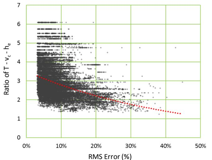
Fig 5. Model error in relation to  $v_c$  and  $h_e$  and  $T$ . Each Colding model is represented with (●) and an exponential curve fit of the average ratio for any specific model error is represented with (●).
