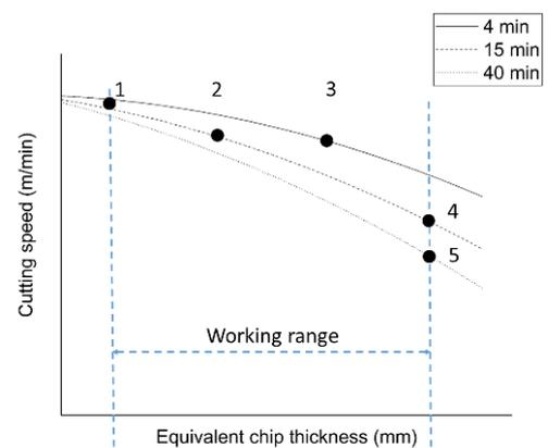
Fig 8. . Suggestion on placement of the cutting data points in a test series of five tests.
